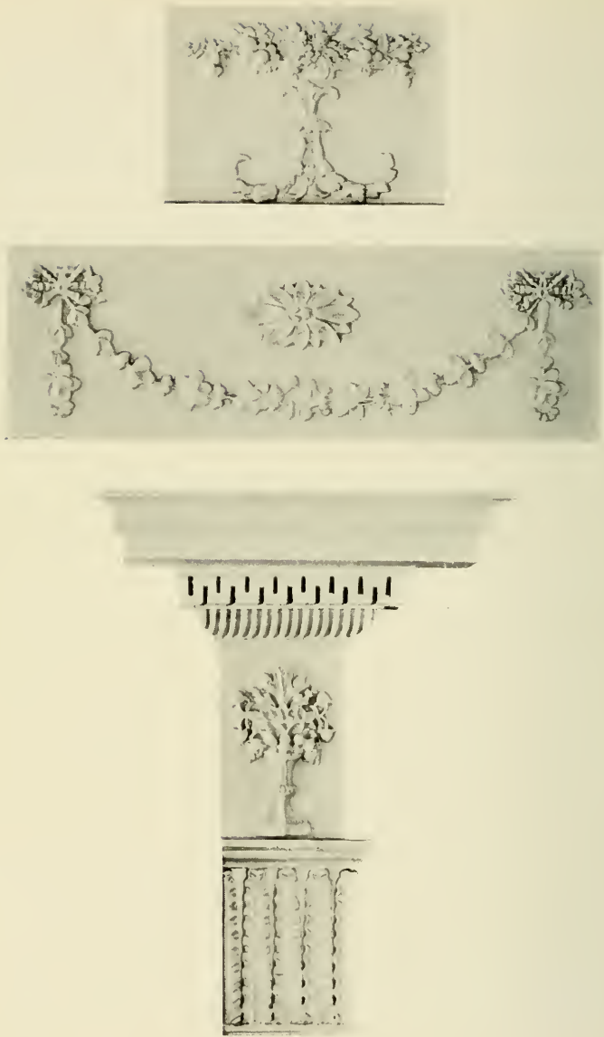
PLATE CIX.—Detail and Corner Section of East Parlor Doorway, Pierce-Johonnot-Nichols House.
